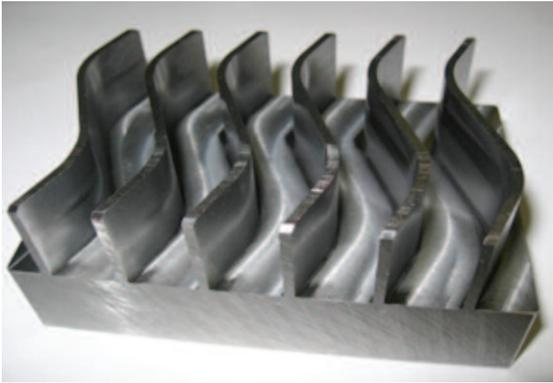
Cutting narrow slots in hardened steel has long been one of the most difficult machining tasks - and one that OKK, Union Tool and DP Technology teamed up to solve.
